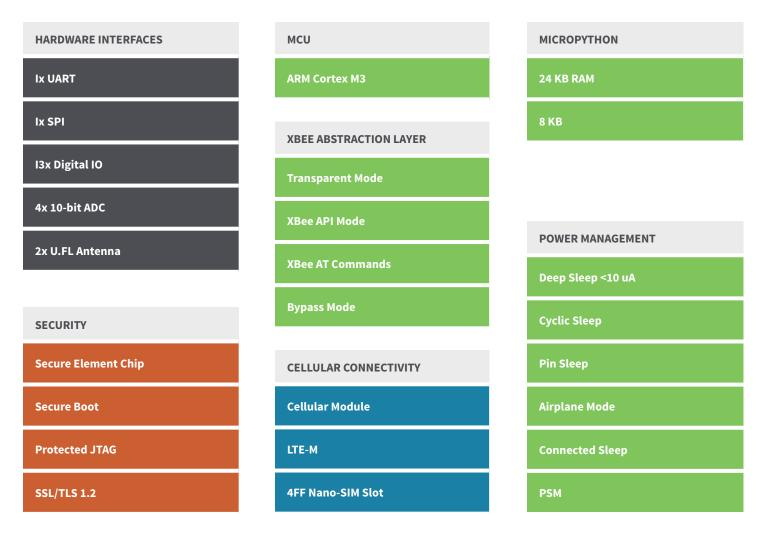
**Digi XBee 3 software interface** — The Digi XBee 3 software interface runs on the onboard microcontroller and provides an abstraction layer for software designers, including a common AT command interface for configuration and control, an API mode for external devices to intelligently communicate with the XBee, and a transparent serial mode for simple and transparent communications through the UART, over the cellular network, to the destination IP address or phone number.
