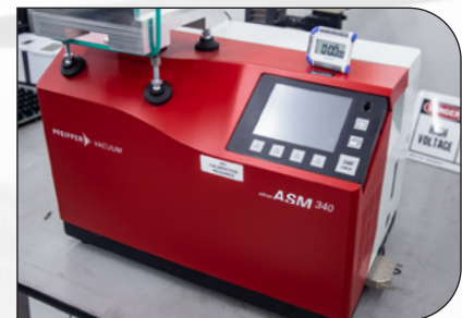
Fine leak testing
