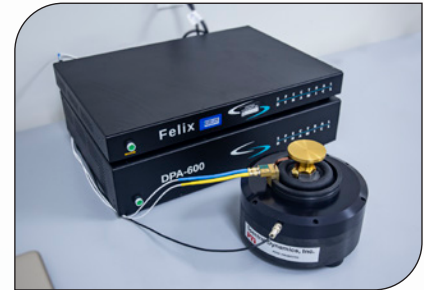
Particle Impact Noise Detection (PIND)
