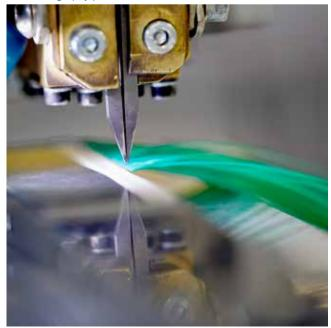
Welding of wires to the sensor
