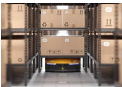
**AGVs**, such as tractors or automatic forklifts, need to be equipped with a variety of sensors: CAN Bus is used as the communication interface of the infrared distance measuring device to detect pallets, avoid collisions during navigation, and position the fork
