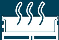
Adding a *Heat Spreader* enhances the DRAM module's ability to quickly disperse heat in high-temperature and heavy workload environments. Innodisk's heat spreaders are compatible with all form factors and help ensure that temperatures stay below the critical limit where module failures start occurring. By reducing thermal stress, heat spreaders also extend the lifespan of DRAM modules.
