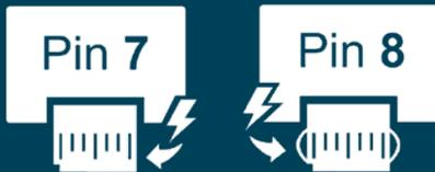
Innodisk's patented Pin 7 and Pin 8 SATA power technologies take the cable-less concept to the next level by eliminating the need for power cables. The result is a 100% cable-less, shock-resistant, space-saving, and plug-and-play storage solution. Innodisk's cable-less power solutions mean optimized airflow and optimal use of the limited space in embedded and rackmount server systems.
