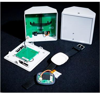
The tags are the devices being tracked. Depending on the use case, being indoor, outdoor, nature of tracked item and the level of IoT functionality required, these form the customised element of any solution.
